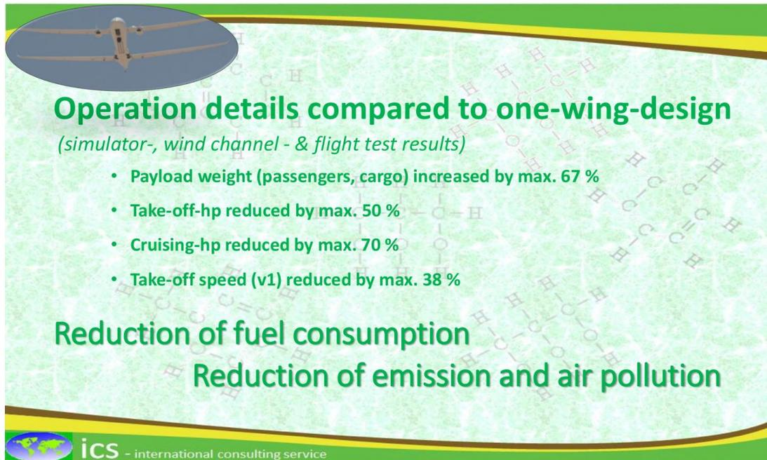
**Operation details compared to one-wing-design**
